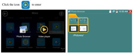
The Media player can browse video and image files. It supports the video formats of MP4, H.264, MPEG4 and MKV. The IP tester recorded files can play directly via the Media player. The Media player will automatically display the video files from the SD card. Click on the desired file to play. Click RETURN to exit.
