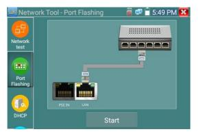
If the tester and PoE switch are connected well, the LAN port of POE switch flash at special frequency, If not, no any changes on the LAN port
