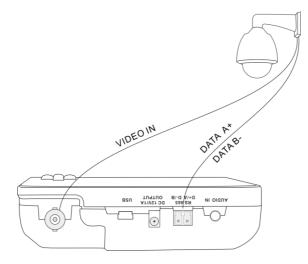
(1) Connect the camera's video output to the IP tester's VIDEO IN. The image will display on the tester after pushing the PTZ icon
