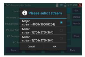
**IP Camera's IP:** Enter the IP camera's IP address manually or click "Search" to auto-scan for the IP camera's IP address. It is better to directly connect the IP camera to the tester so the search results will only display the camera's IP address. If the tester is connected to a PoE switch, it will find and display several IP address
