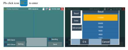
Click "Setting" to choose the baud rate of RS485; it must be the same as the DVR or the Control keyboard. The DVR or Control keyboard send the code to the tester, if it can be read, the protocol will shown on the upper right, like Pelco D, if not, like P:---
