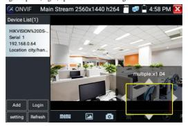
If it is network video input to the tester, as the tester supports resolution up to 1080p, the input image will be very clear after it is enlarged. This is greatly helpful for the installers to ensure the IP camera's video coverage and decide the IP camera's install site.
