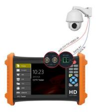
(1) Connect the SDI camera's video output to the cctv tester's "SDI IN" interface, the image will display on the tester. The tester only come with SDI input interface. There is no SDI output interface.
