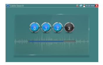
Use the blue Combination cable identifier and network cable tester's copper pointer to touch all the cables in the bundle.
