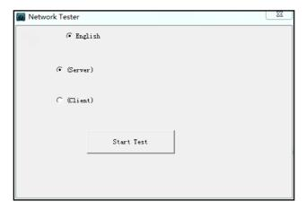
Tester as Client, tester's IP address is:192.168.0.238. The Server and the Client are at the same network segment, but with different IP address. Input Server's IP address 192.168.0.39 in the tester and click "Start" to test network bandwidth.
