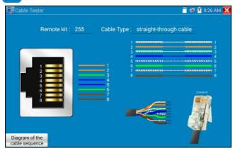
Test LAN cable or telephone cable.
