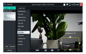
When the image is enlarged, if not operate on touch screen, it can operate by the keyboard, press the key to zoon in, press the key to zoom out, press upward and downward key to move image.
