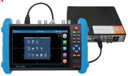
DVR or other device's HDMI out port connect to tester's HDMI in port, the meter will display input image.
