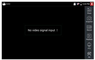
When AHD signal input, the tester will display the image resolution on the top bar. Double-taps on the screen to make the image displayed full screen.
