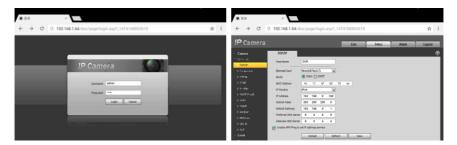
The IP camera and IP tester be on the same network segment for the browser to interface with the camera. If they are not in the same segment, click the button (RETURN) or press "RETRUN" to exit. Open the "Settings" app from the main menu to change the IP tester's network settings to match those of the IP camera.
