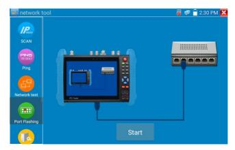
If the tester and PoE switch are connected well, the LAN port of POE switch flash at special frequency, If not, no any changes on the LAN port
