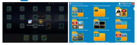
The Media player can browse video and image files. It supports the video formats of MP4, H.264, MPEG4, and MKV. The IP tester recorded files can play directly via the Media player. The Media player will automatically display the video files from the SD card. Click on the desired file to play. Click RETURN to exit.
