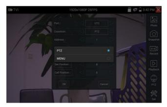
Input calling dome camera menu address code, after finishing the parameter settings, you can press the key (ENTER) or click the icon to call the dome camera menu.
