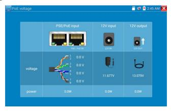
Warning: Not allow connect device with input power over 17V to tester "12V IN" port, otherwiseit will damage the machine.
