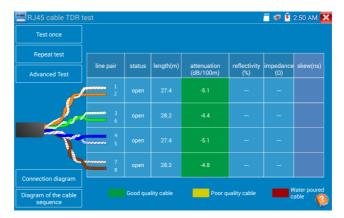
**Advanced Test:** Test cable pair status, length, attenuation, reflectivity, impedance, skew and other parameter.
