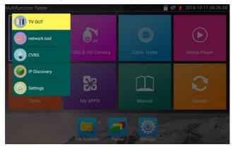
Press the key" (MENU)", you can turn on it, and switch functions, then press (1) to enter app, tap other area on the screen, to exit the menu.
