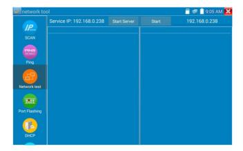
When test, need a tester or a computer installed Network Test Software as the Server, the other tester sends packet test. The two testers must be in the same network segment.
