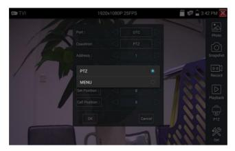
Input calling dome camera menu address code, after finishing the parameter settings, you can press the key  $\overbrace{\text{enter}}$  or click the icon  $\overbrace{\text{to call the dome camera menu}}$ .
