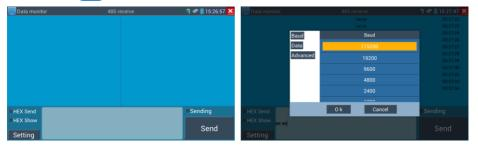
Click "Setting" to choose the baud rate of RS485/RS232; it must be the same as the DVR or the Control keyboard. The DVR or Control keyboard send the code to the tester, if it can be read, the protocol will shown on the upper right, like Pelco D, if not, like P:---
