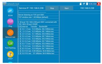
**b). Start send packet test:** Using the other IP tester, type in the Server's IP address at the top right corner of the screen. This app is used to send packets for network speed testing. Click the "Start" button to send the packets and start testing.
