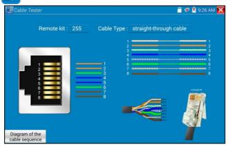
Test LAN cable or telephone cable.
