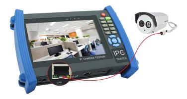
Note:1) If the IP camera requires PoE power, then connect the IP camera to the IP tester's LAN port. The tester will supply PoE Power for the IP camera. Click on the icon labeled POE to turn the PoE Power off or on.
