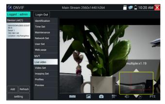
When the image is enlarged, if not operate on touch screen, it can operate by the keyboard ,press the key to zoom in , press the key to zoom out ,press upward and downward key to move image.
