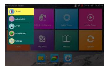
Press the key" MENU", you can turn on it, and switch functions, then press ( to enter app, tap other area on the screen, to exit the menu.
