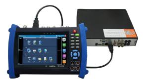
DVR or other device's HDMI in port connect to tester's HDMI in port, the meter will display input image
