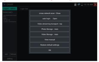
Across network segments scan: After open this function, enter "Setting"-"IP Settings"-"Advanced" to add other network segments IP, Rapid ONVIF function can across network segments to scan camera's IP.
